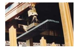
• Special recommendation for the use of electro-permanent magnets is made for locations where sudden interruptions of main electrical power may happen inadvertently.
